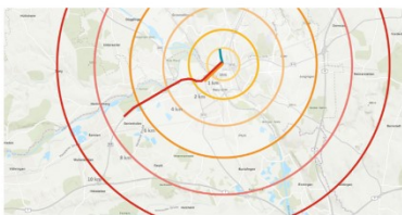
Bauphase 1 ca. 3610 Kfz/h resultieren in ca. 9,6 km Stau (FR-Nord)
